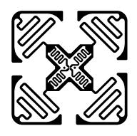
This antenna is designed for logistics applications. It supports omnidirectional reading, and its high efficiency and excellent performance make it widely used in warehouse management, logistics and transportation fields etc. The deployment of RFID technology in warehouse management and logistics transportation will help monitor the flow direction of products and ensure the safety of cargo transportation.
