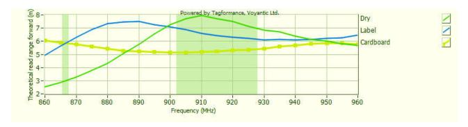
Sensitivity&Read Rang Test power: 4W EIRP
